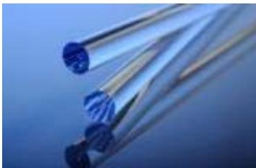
Photo caption no. 222781: Long rods made of optical glass: With diameters of < 1 mm and lengths of up to 1000 mm, the long rods made of specialized optical glasses from SCHOTT (low Tg glasses, LASF35, etc.) that feature a fire-polished surface are used for manufacturing miniaturized optical components.
