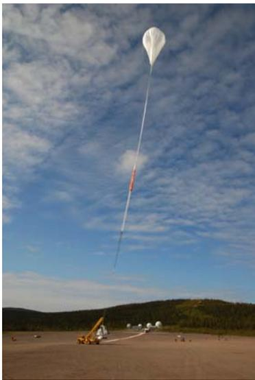
Caption no. 227905: "Sunrise" at the arctic circle: "Sunrise", the solar observatory attached to the helium-filled balloon lifts off from the European Space Center "Esrange" near Kiruna in northern Sweden. "Sunrise" carries the largest solar telescope ever to leave ground. On board: the lightweight 1.1m primary mirror made of the glass ceramic "Zerodur" from SCHOTT.
