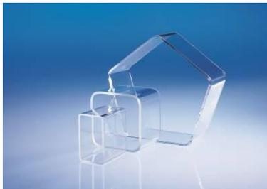
Photo no. 30660, 30662, 30663: Conturax Pro: SCHOTT manufactures angular profiled tubes using a patented, direct drawing method. The tubes can be used in a number of different ways, for instance product design, for lighting, architecture, plant construction, in addition to other technical applications. Source: SCHOTT
