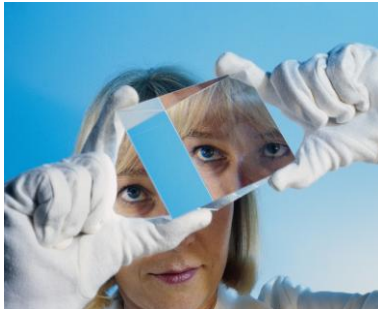
Photo no. 21440: SCHOTT developed the highly transparent glass N-BK7HT for use in manufacturing homogenous optical components in which light travels long distances, such as prisms, for example. Source: SCHOTT
