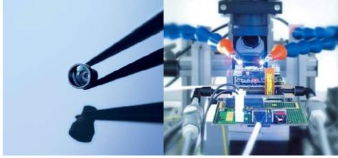
**Photos:** FISBA develops and manufactures customized optical microsystems for use in Life Sciences or machine vision applications, for example. The illumination lens shown here is part of a 3-D scanner featuring 18 optical elements. This miniature visualization system for measuring complex cavities is only 3.6 mm in diameter and slightly less than 20 mm long. Source: FISBA OPTIK AG.
