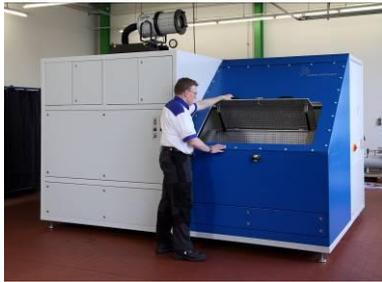
Image: Poppe + Potthoff has developed a burst pressure test stand for hydraulic components for and in cooperation with Eaton. This machine tests tube couplings and hose assemblies in a massive test chamber up to bursting. The hydraulic aggregate is operated from the PC station via Eaton's XC200 controller. The system is connected to the graphic programming environment of National Instruments (LabVIEW) and the local network via an integrated interface.
