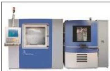
Fig. 1: With a new pressure pulsation test stand Poppe + Potthoff Maschinenbau GmbH enables comprehensive testing of medium transporting components according to all strict test standards of the German automobile industry.
