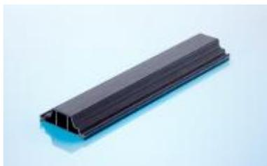
*Fig. 4: Dust blasting the insulbar ESP insulating profile - recognizable by its matt, slightly roughened surface - increases the surface tension of the polyamide bar, guaranteeing durable paint adhesion.*
