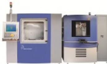
Photo 2: Vacuum impulse pressure test stand for plastic components: Poppe + Potthoff Maschinenbau allows for positive and negative pressure testing of 0.5 to 2 bar and 1 to -0.8 bar under changing temperatures in a climatic chamber.
