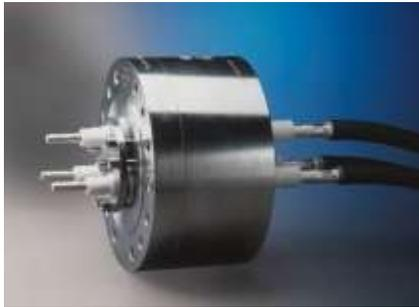
Double-sealed Eternaloc® terminal header assembly from SCHOTT: The conductors are insulated with two separate glass-to-metal sealed flange modules that are hermetically connected and form a compact double barrier that offers superior safety features on par with electrical penetrations designed for nuclear power applications. Source: SCHOTT
