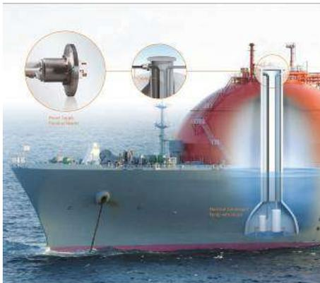
In order to unload liquefied gas, the storage tanks on board an LNG tanker contain powerful electric pumps. The pumps and their motors are mostly integrated into a chassis and work completely immersed in liquefied gas. SCHOTT's terminal header assemblies serve as the hermetic feedthroughs for the three-phase electrical power, as well as the control and instrumentation signals. Source: SCHOTT
