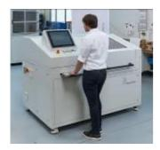
Photo 1: The burst pressure test stand for plastic components from Poppe + Potthoff Maschinenbau enables a high-precision and fast component test.
