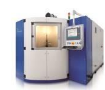
Fig. 3: This test stand by Poppe + Potthoff Maschinenbau produces strong impulses up to 6,000 bar with a frequency between 1 and 30 Hz to check the durability and strength of components under pulsating inner pressure.
