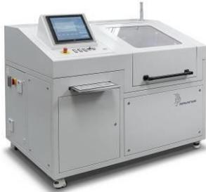
Photo 1: The burst pressure test stand for plastic components from Poppe + Potthoff Maschinenbau enables high-precision and fast testing.
