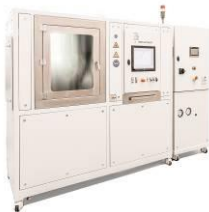
Fig. 4: The Poppe + Potthoff Maschinenbau function test bench measures the energy consumption and performance data of heating and cooling units under changing temperature conditions so that their efficiency can be optimized.
