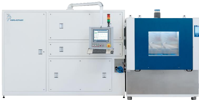
Fig. 1: Components for liquid-cooled systems in data centers are tested with the pressure cycling test bench from Poppe + Potthoff Maschinenbau.
